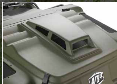
VENTED HOOD FOR IMPROVED ENGINE COMPARTMENT COOLING
