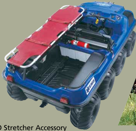
ARGO Stretcher Accessory fits all current ARGOn 8x8 models and is designed for Ferno Stretcher #9.
